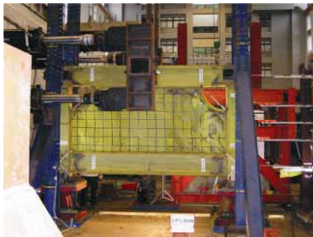
Figure 1: SPW Specimen with Cutout Corners to Accommodate Nonstructural Systems.
